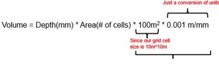
Volume = Depth(mm) \* Area(# of cells) \* 0.1 m<sup>3</sup>/mm
