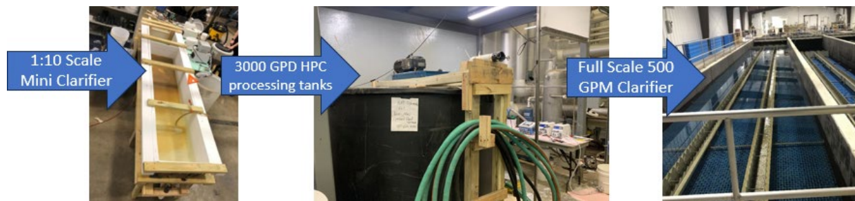
Figure 5. Photos (shown left to right) of 1:10 scale upstream concentrator test unit, 1000-gallon batch reactor for generating both first and second spilt pH, and full-scale upstream concentrator located at A-34.
