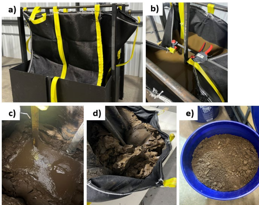
Figure 72. 400-gallon geobag performance test C1: a) hanging bag; b) bag following Charge 1; c) HPC dewatering after three charges and one week of drainage; d) HPC after 57 days of indoor drying; e) HPC after two additional months of outdoor drying.
