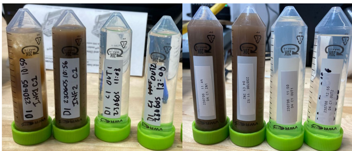
Figure 76. Typical influent and effluent samples from short-term storage tests: test D1, flocculated in clarifier (left); test D4, flocculated at pump (right).
