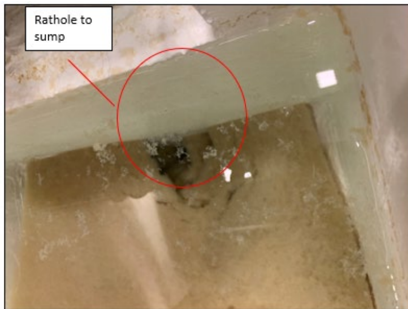
Figure 36. “Rat holing” to sump on A-34.
