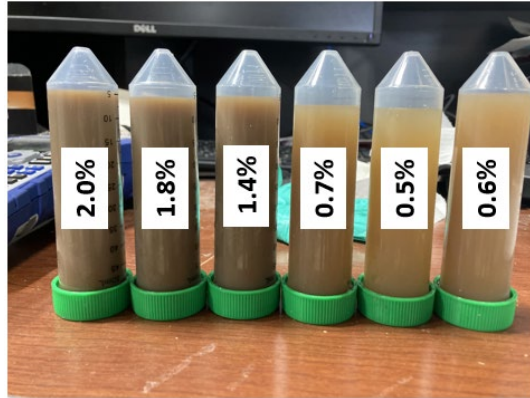
Figure 81. Typical variation in total solids when pumping form Clarifier 2 to geotube E1.
