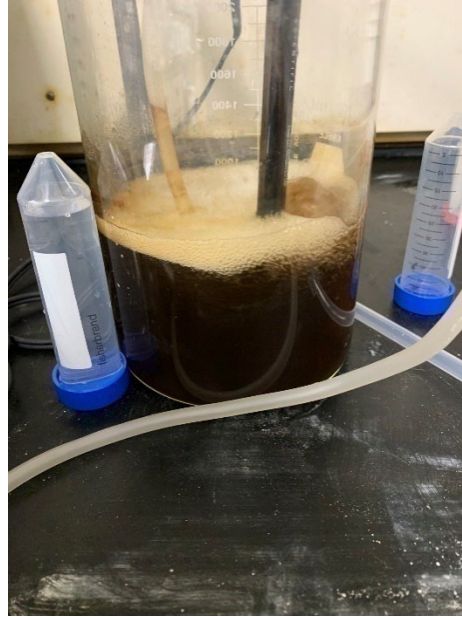
Figure 40. Ozone precipitating solid from neutralized raffinate solution.
