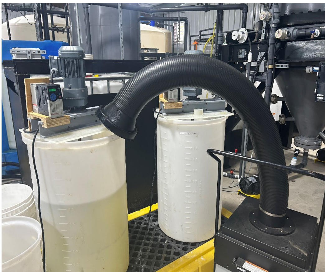
Figure 16. 55-gallon capacity stripping circuit.
