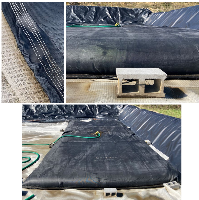
Figure 82. Photos of geotube E1 (clockwise from top left): clear filtrate during pumping, front view at end of performance period, full view at end of performance period.
