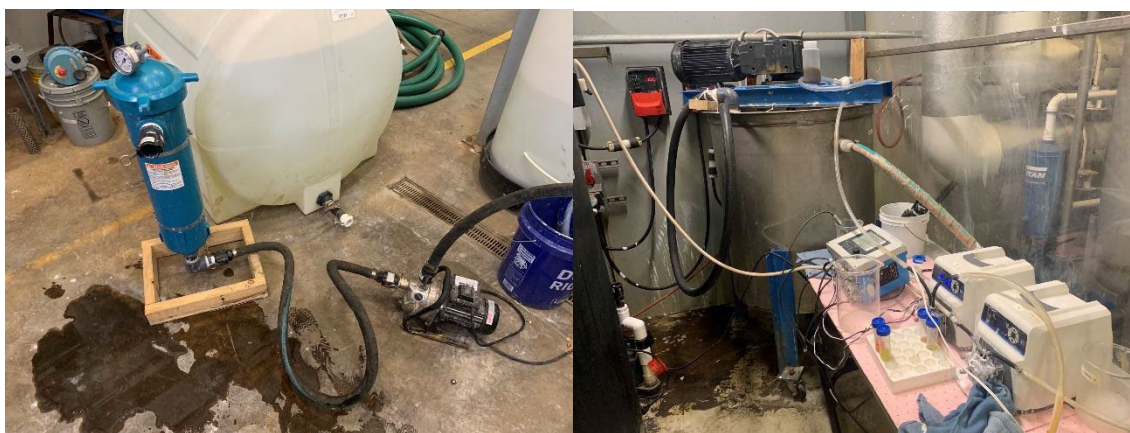
Figure 27. Left: Filter house and pump used to separate PLS from leaching residuals. Right: Vat, pumps, and automated pH controller used to leach HPC and neutralize PLS.
