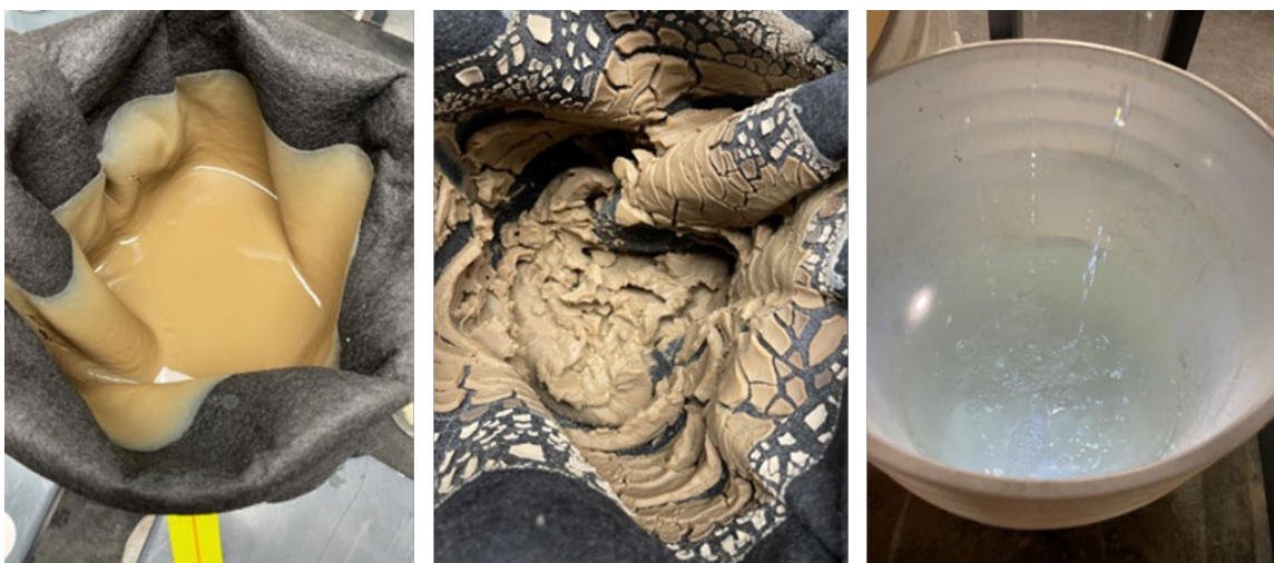
Figure 67. Mini bag test execution (from left to right): retained HPC during filling; retained filter cake after filling and drainage; filtrate during bag filling.
