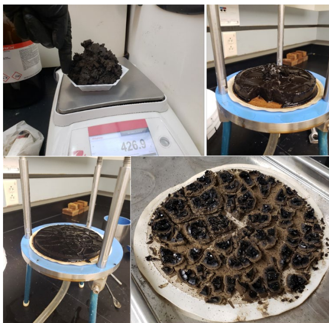
Figure 18. (Top Left) Initial Wet PC (Top Right) Residue after first filtration (Bottom Left) Solid residue after second filtration (Bottom Right) Dried residue.
