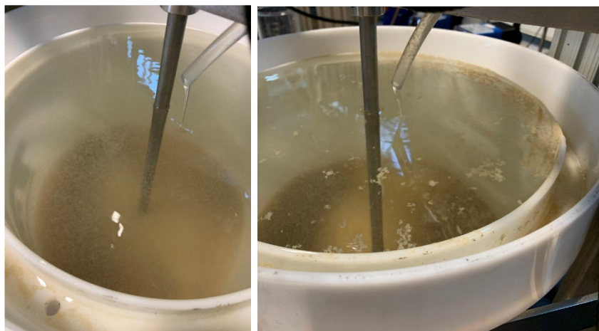
Figure 4. Operation of bench-scale clarifier (left) without addition of flocculant, and (right) addition of flocculant.
